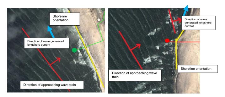
Wave train approaching the proposed southern discharge site. Note the approaching wave train is approximately parallel to the shoreline orientation. Wave train approaching the proposed northern discharge site. Note the approaching wave train is oblique to the shoreline orientation.
