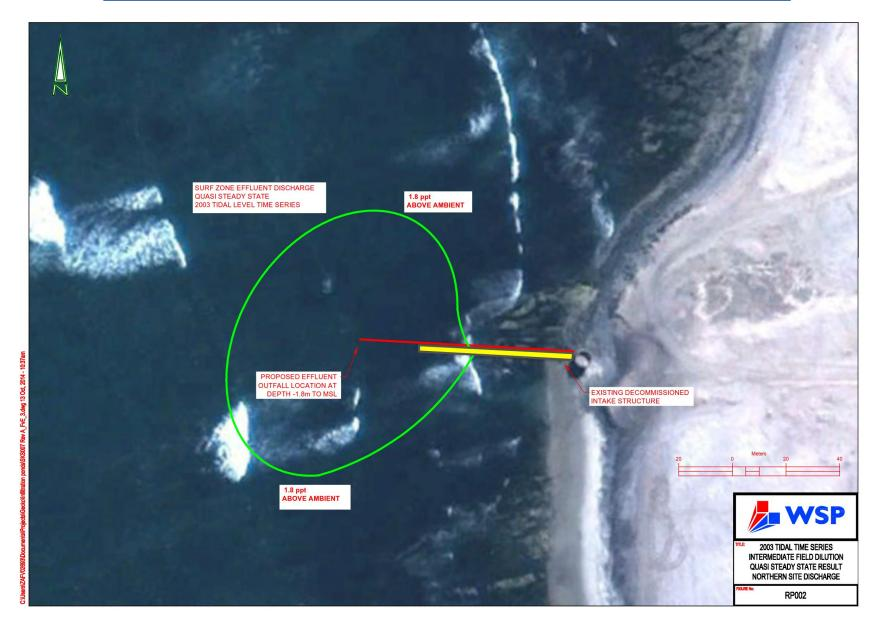
Drawing RP002: Contour plot of the diluted intermediate field brine influence area (given in parts per thousand above ambient salinity) for the northern site.
