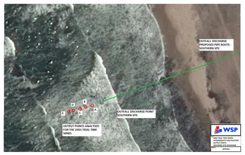
Drawing RPRT001: Locations of output points analysed for the 2003 time series. The points are spaced 5m apart with point E being 22m from the point of initial dilution.
