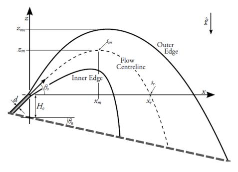
Figure 3.1: Configuration and notation for an inclined negatively-buoyant jet (Oliver, 2012)
