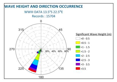
Figure 4.2: Wave rose of the ten year data set indicating wave direction and percentage occurrence of wave heights
