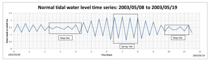
Figure 6.1: Normal tidal water level time series: 2003/05/08 to 2003/05/19 representing the average wave conditions occurring at the site.
