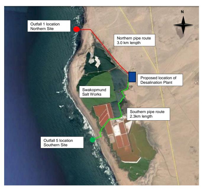
Figure 2.1: Layout of site and location of proposed and two outfall sites considered
