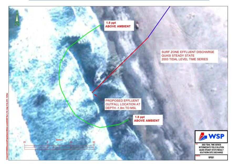
Drawing RP001: Contour plot of the diluted intermediate field brine influence area (given in parts per thousand above ambient salinity) for the southern site.
