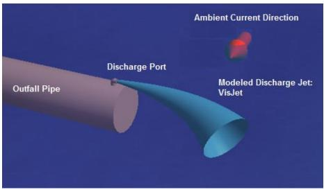
Figure 5.1: VisJet model rendering of an outfall jet. The blue cone simulates the evolution of the discharge jet over distance. The red arrow indicates the current direction. Note that the pipe size rendering is exaggerated.
